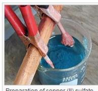
Preparation of copper (II) sulfate by electrolyzing sulfuric acid, using copper electrodes
